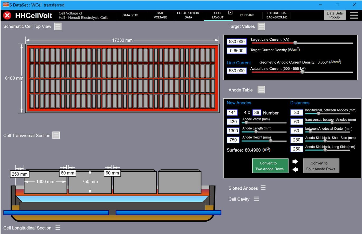
Figure 1: HHCellVolt layout of the wide cell design using 36 anodes, each having 4 carbon blocks
