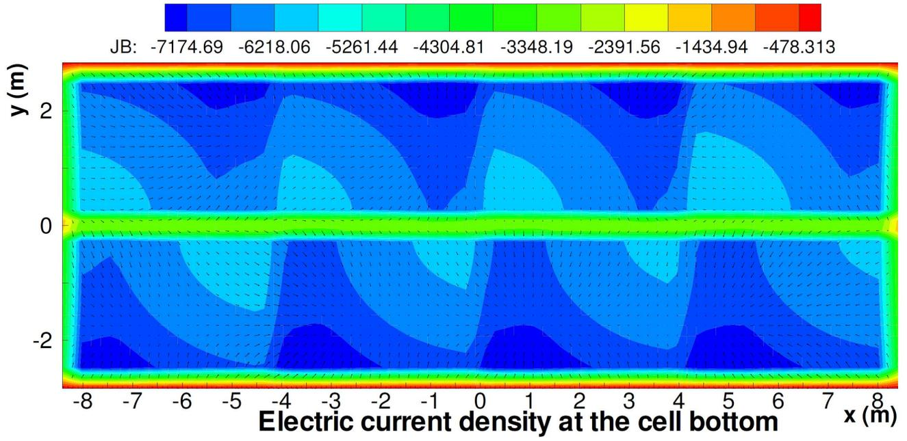
Figure 3: Cathode surface current density and mid metal pad horizontal current
