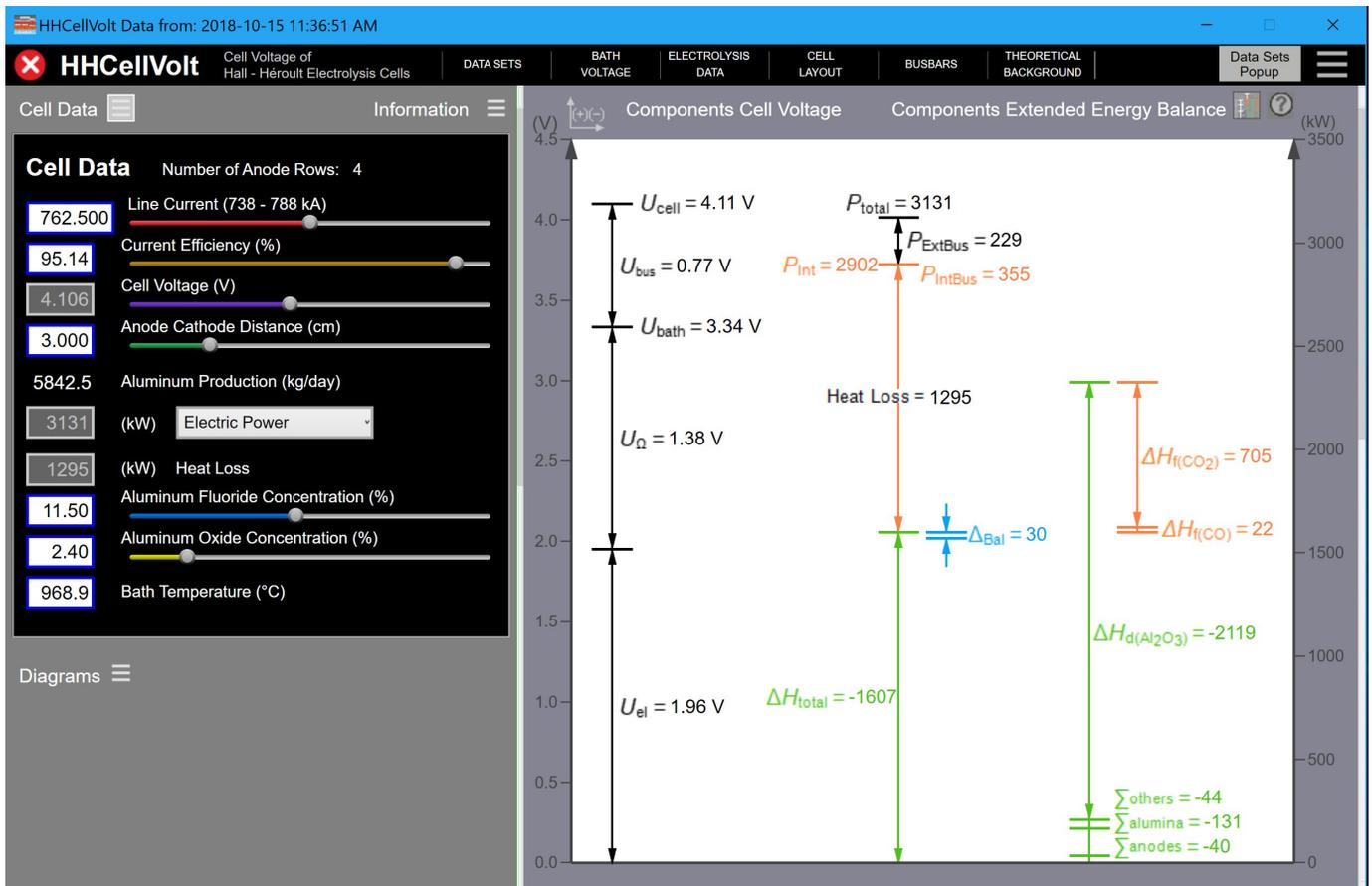
Figure 2: HHCeIVolt main results for the initial wide cell design operating at 762.5 kA
