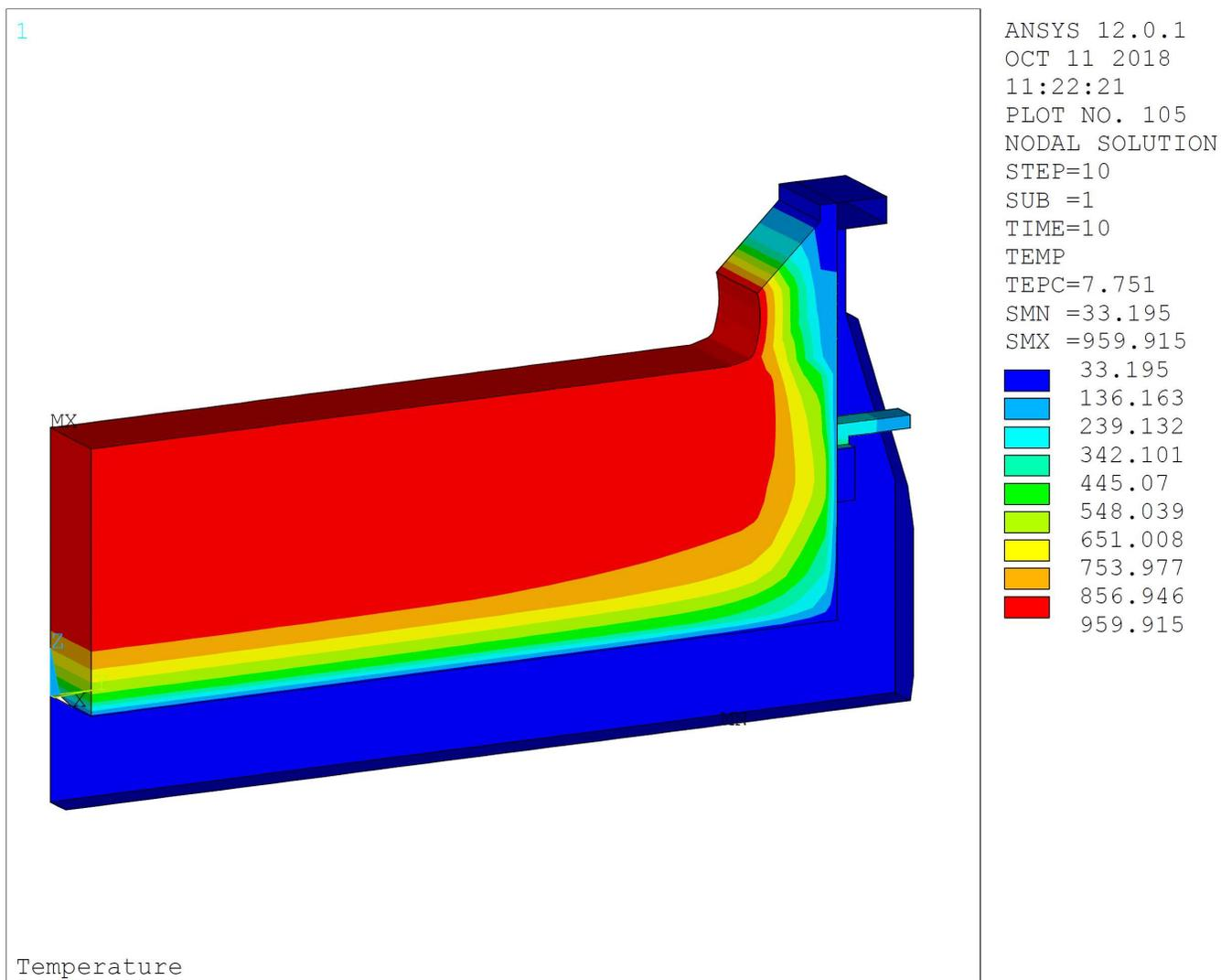
Figure 7: ANSYS based cathode side slice thermo-electric model isotherms with converged ledge profile
