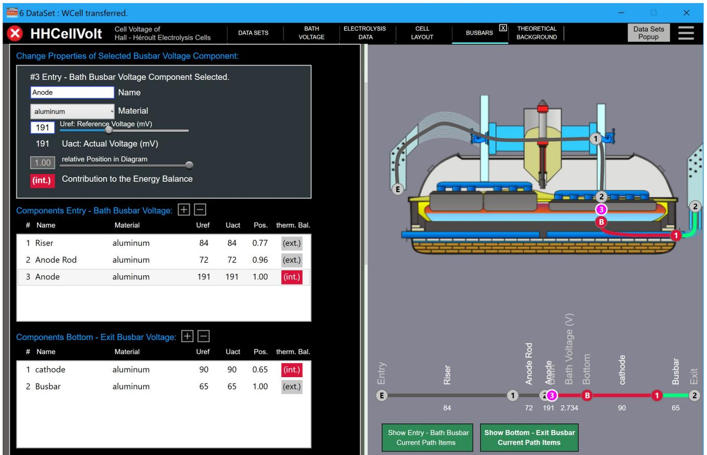
Figure 8: HHCeIVolt barbars voltage drop input panel
