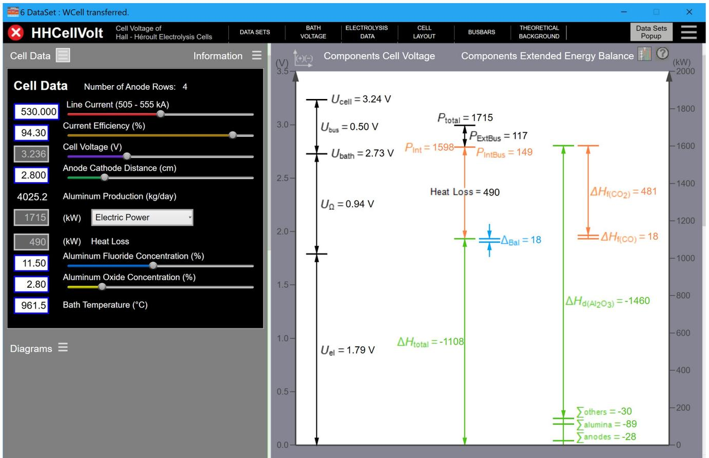
Figure 10: HHCeIVolt main results for the final wide cell design operating at 530 kA
